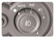
The Fog Lamps button is located in the center of the exterior lamps control ("A" above). Press it to activate or deactivate fog lamps.
